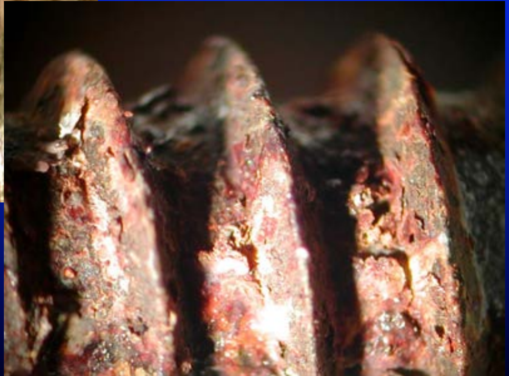
Screw Threads - 1537 Cycles
