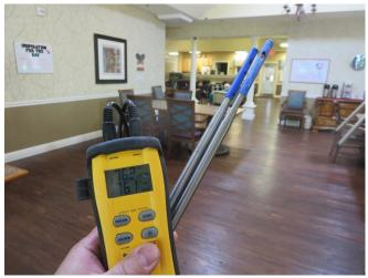
Figure 2: Dual in-duct psychrometer
