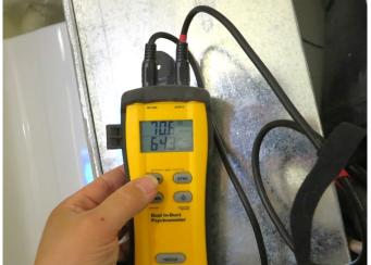
Figure 13: Measuring "split" across an AHU
