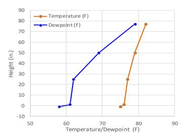
Figure 11: Direct measurement of unvented attic thermal and moisture stratification
