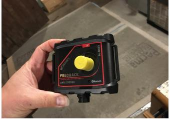
Figure 3: Tramex DL-RHTX T/RH meter
