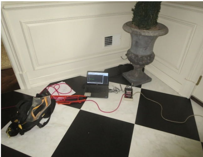
Figure 10: Using TECLOG to log pressures
