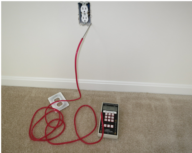
Figure 7: Measuring \Delta P at an electrical outlet
