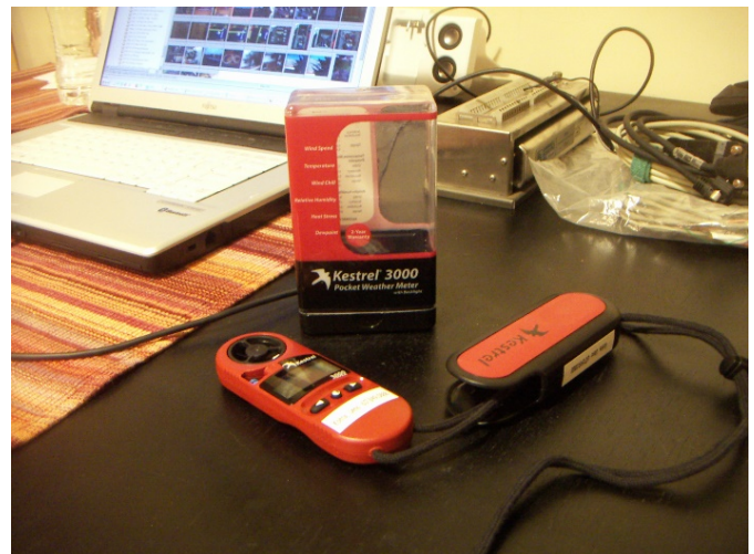
Figure 13: Kestrel wind (air velocity) meter
