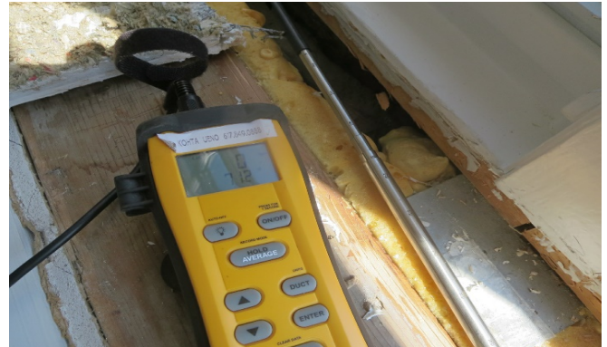
Figure 15: Hot-wire anemometer air velocity meter
