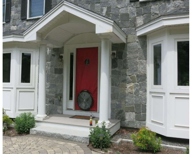
Figure 1: Testing a house with a blower door
