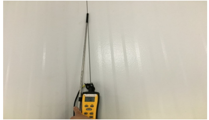
Figure 14: Hot-wire anemometer air velocity meter
