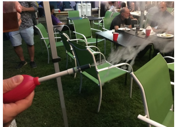
Figure 12: Smoke pencil from a vaping pen
